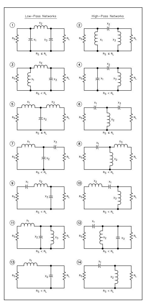
This page accompanies the ARRL Handbook software package that is available at http://www.arrl.org/notes/. This figure shows the 14 possible network configurations used by NBMATCH.BAS. Refer to this figure and enter the desired network by number when you run the program. Note that low-pass networks have an odd identifying number while high-pass networks have an even identifying number. See the Network Equations section of Chapter 17.
