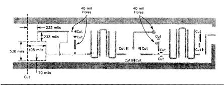
Fig 5—Cutting and drilling guide for the Teflon microwave board.
