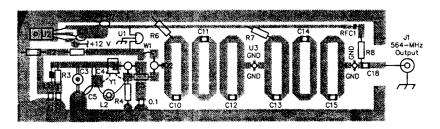
Fig 7—Parts-placement diagram for the 564-MHz local oscillator board.
