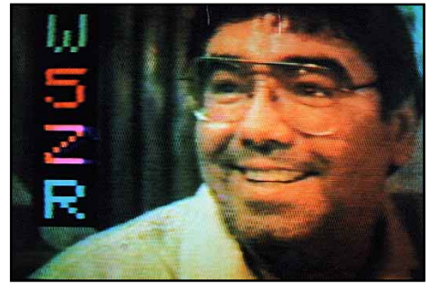
An SSTV image as seen on a standard TV set using a digital scan converter.
