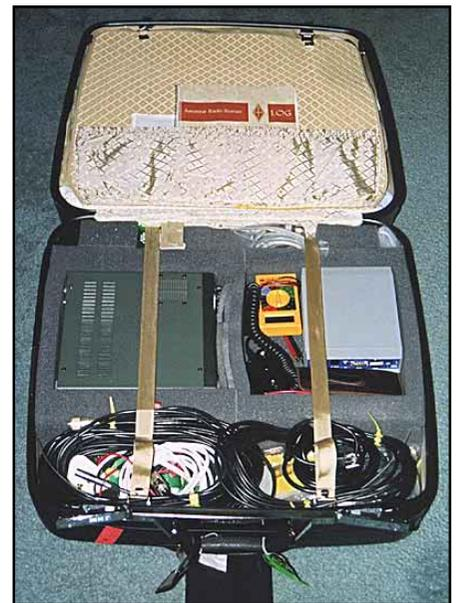
**This suitcase houses a complete portable PACTOR station: transceiver, PACTOR controller, wire antenna and cables, all in one convenient package. Its owner, Joe Mehaffey, K4IHP, of Atlanta, Georgia, connects it to his laptop computer to operate mobile or from almost anywhere he pleases. He even used it to maintain a regular schedule with ham family members and neighbors while traveling around the Australian countryside. (photo by K4IHP)**
