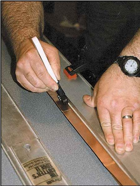
**Fig 11.38**—Larry Wolfgang, WR1B, using a 4-foot straightedge designed as a guide for hand-held circular saws to clamp the copper foil tape to a board on a tabletop. After carefully measuring to ensure a uniform 22 mm width, he cut the foil tape using a Fiskars rotary cutter. Be careful to keep the cutter wheel against the straightedge for the entire length. Move the tape in 4-foot intervals to cut the entire length. (Photo by Dan Wolfgang.)
