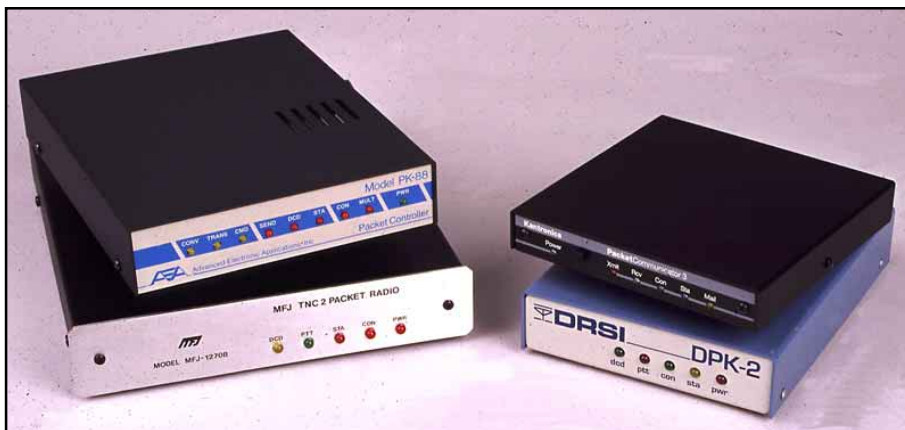
Fig 12.29 —Four popular 1200 bit/s packet TNCs: (clockwise, from bottom left) the MFJ-1270C, AEA PK-88, Kantronics KPC-3 and the DRSI DPK-2.
