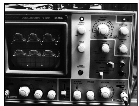
Fig 12.66—An oscilloscope used to observe a video waveform. The lower trace is the video signal as it comes out of the sync stretcher. The upper trace is the signal from the Mirage D1010-N amplifier.
