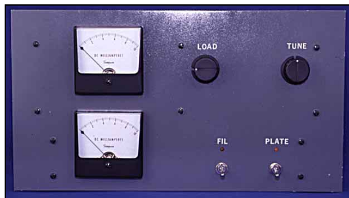
Fig 13.37 —Photo of the front panel of W1QWJ’s 6-meter 4CX1600B amplifier.
