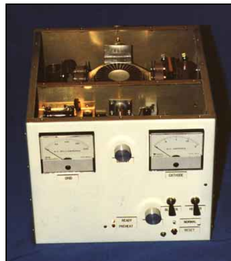
Fig 13.44—This table-top 2-m power amplifier uses a quick-warm-up tube, a real plus when the band suddenly opens for DX and you want to join in.
