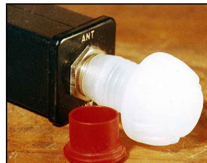
Fig A —Champagne corks may be recycled into protective caps for SO-239 connectors.
