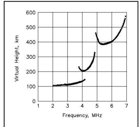
**Fig 21.7**—Gradual refraction in the ionosphere allows radio signals to be propa-gated long distances. It is often convenient to imagine the process as a reflection with an imaginary reflection point at some virtual height above the actual refracting region. The other figures in this chapter show ray paths as equivalent reflections, but you should keep in mind that the actual process is a gradual refraction.
