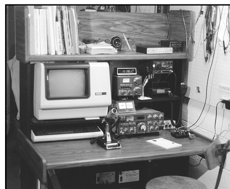
Fig 22.4 —The basement makes a good location if it is dry. A ready-to-assemble computer desk makes an ideal operating table at a reasonable price. This setup belongs to WK8H. (Photo courtesy AA8DX)
