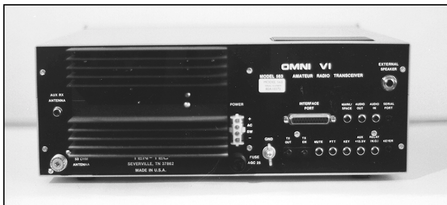
Fig 22.10 —The back of this Ten-Tec Omni VI HF transceiver shows some of the many types of connectors encountered in the amateur station. Note that this variety is found on a single piece of equipment. (Photo courtesy AA8DX)
