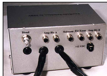
Fig 22.82 —A view of the rear panel of the main box of the Two-Radio Switchbox.
