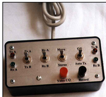
Fig 22.83 —The remote head for the Two-Radio Switchbox.
