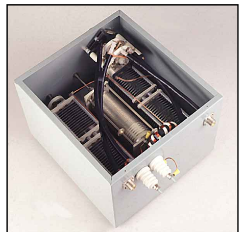
Fig 22.96—Interior view of the ARRL Antenna Tuner. The balun is mounted near the input coaxial connector. The two feedthrough insulators for balanced-line operation are located near the output coaxial unbalanced connector. The Radioswitch Corporation high-voltage switch is mounted to the front panel. Ceramic-insulated shaft couplers through ground 1/4 -inch panel bushings couple the variable components to the knobs.
