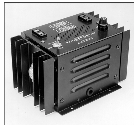
Fig 22.34—Photograph of a commercial dc-to-ac inverter that operates from 6 to 12 V dc and delivers 120 V ac (square wave) at 175 W.
