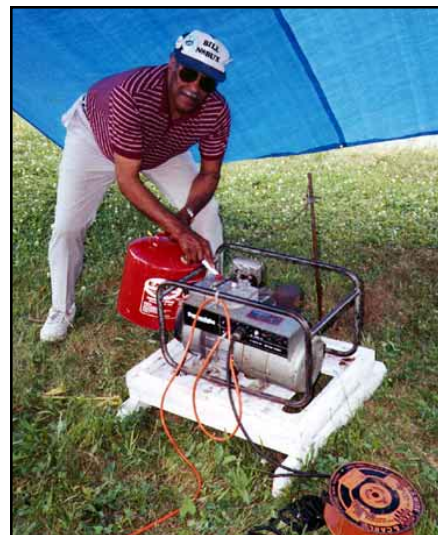
Fig 22.35—Modern gasoline engine-powered generators offer considerable ac power output in a relatively compact and lightweight package.
