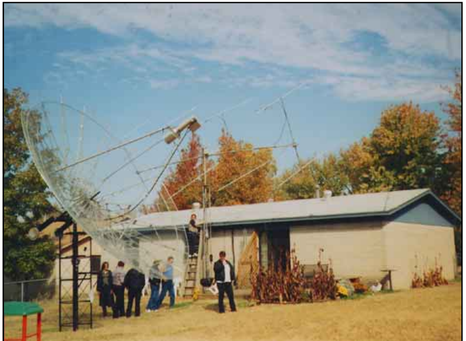
Tommy Henderson, WD5AGO, pursues 144-MHz EME from his Tulsa, Oklahoma, QTH with this array. Local electronics students helped with construction.
