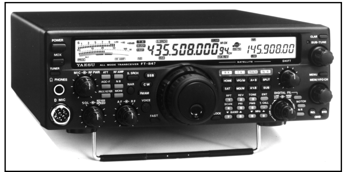
The Yaesu FT-847's satellite mode provides the user with a full featured satellite transceiver. As a bonus, it also covers all the HF bands!
