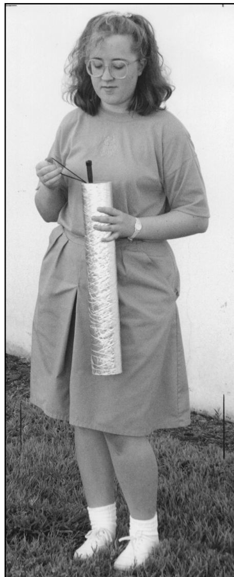
Fig 23.90 — The air attenuator for a VHF hand-held in use. Suspend the radio by the wrist strap or a string inside the tube.
