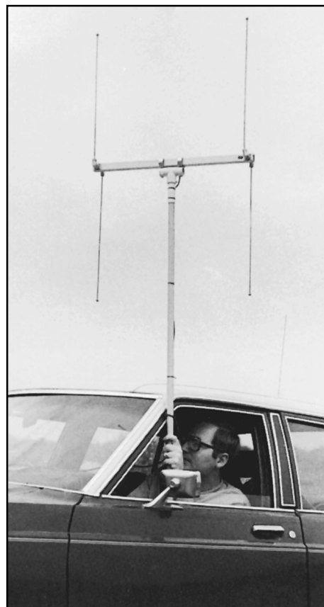
Fig 23.84 — A set of TDOA RDF antennas is light weight and mounts readily through a sedan window without excessive overhang.
