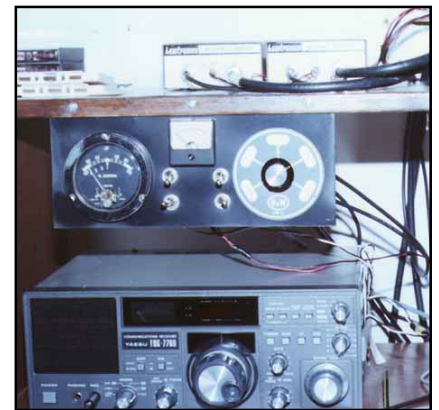
Fig 23.39 — An entry-level receiving station using 2 m and 70-cm converters and a general coverage communications receiver.
