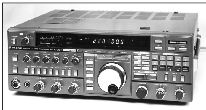
The Yaesu 736R is a multimode transceiver for 2 m (144-148 MHz) and 70 cm (430-450 MHz). It can be used for full-duplex receiving and transmitting on AO-10 Mode B and AO-13 Modes B and J. An optional 23-cm module covers 1230-1300 MHz (Mode L). Approximate power output: 20 W on 2 m and 70 cm, and 10 W on 23 cm.
