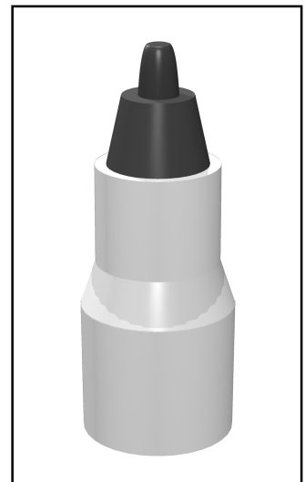
Fig A — Make a permanent marker into a specialized PC-board drawing tool. Simply press the marker point into a drilled hole to form a modified point as shown. More pressure produces a wider shoulder that makes larger pads on the PC board.
