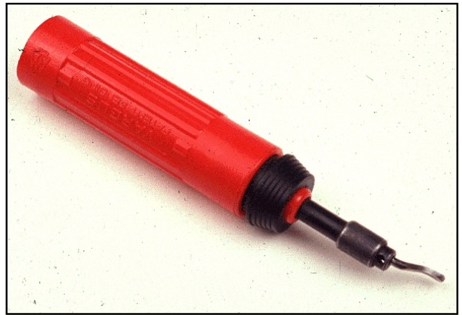
Fig 25.2 — A deburring tool is used to remove the burrs left after drilling a hole.
