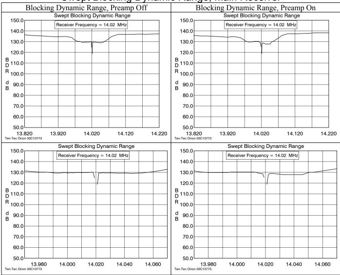
**Note:** In previous expanded reports, the swept graphs were taken with the preamp on, except in the case where a transceiver did not have a preamp (such as the Ten-Tec Omni VI+). This precedent was set with the first expanded reports in 1996. In hindsight, testing all transceivers with the preamp off would have been the more logical choice. For this report, test data is shown for both preamp off and preamp on.
