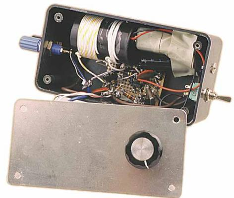
**Fig 1.11 — The art of *homebrewing*, or building your own equipment, is thriving. This small receiver contains two transistors and one integrated circuit. It is assembled without special tools in one or two evenings. The thrill of operating a radio you built lasts a long time! See Chapters 14 and 15 for some receivers and transceivers you can build.**
