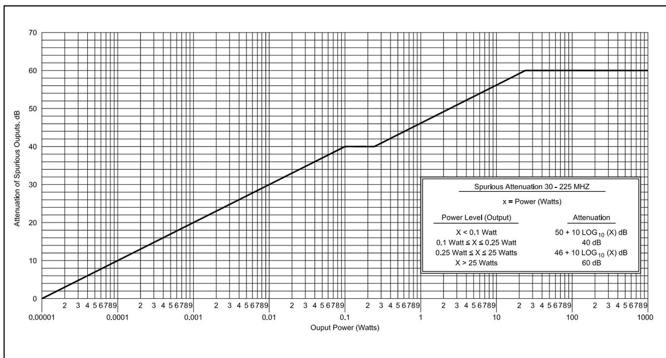
Fig 1.24 — Required attenuation of spurious outputs, 30-225 MHz.
