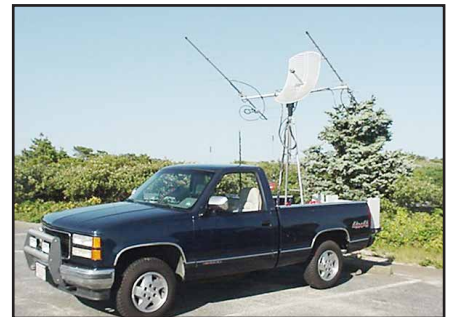
Fig 2.10 — A portable, all purpose, mode V/U/S earth station. This station works LEOs and HEOs (high earth orbiters) like AO-40, and future birds like Eagle. If you live in an area of dense tree growth that impedes your antenna performance, you might consider portable operation at a location with a very low horizon. (photo courtesy of Shawn Reed, N1HOQ).
