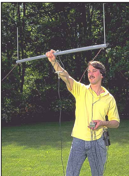
Fig 2.8 — Dave Pingree, N1NAS, hunts down a transmitter on 2-m FM. (photo by Kirk Kleinschmidt, NT0Z)
