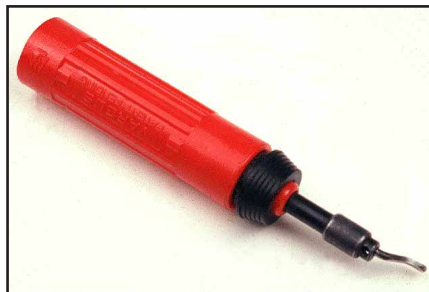
Fig 8.2 —A deburring tool is used to remove the burrs left after drilling a hole.
