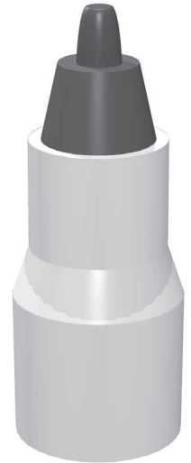
Fig A—Make a permanent marker into a specialized PC-board drawing tool. Simply press the marker point into a drilled hole to form a modified point as shown. More pressure produces a wider shoulder that makes larger pads on the PC board.
