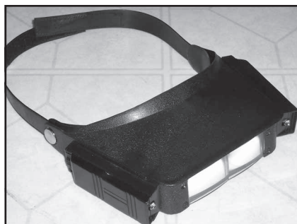
Fig B —A magnifying visor is great for close-up work on a circuit board. These headsets are often available for less than $10 at hamfests and some even come with superbright LEDs mounted on the side to illuminate the components being soldered.
