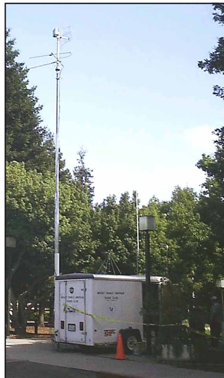
FM voice repeater, amateur television (ATV), and HSMM antennas mounted on a hydraulically operated mast. This portable installation was used to provide shared high-speed Internet access and other special communications support to the many hams attending the 2003 Pacificon Hamvention in San Ramon, CA. The HSMM station is also used to provide streaming video or amateur digital video (ADV) to the Mount Diablo ARC's analog FM ATV repeater on the nearby mountain. (Photo: John Champa, K8OCL)
