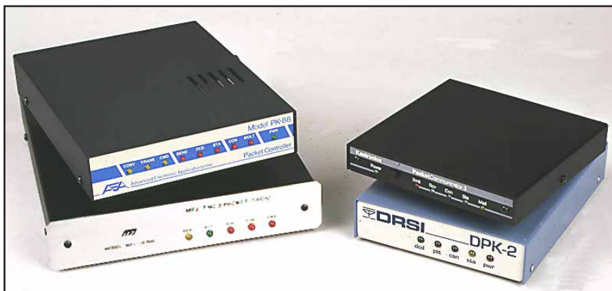
Fig 9.19 — Four 1200 bit/s packet TNCs: (clockwise, from bottom left) the MFJ-1270C, AEA PK-88, Kantronics KPC-3 and the DRSI DPK-2.
