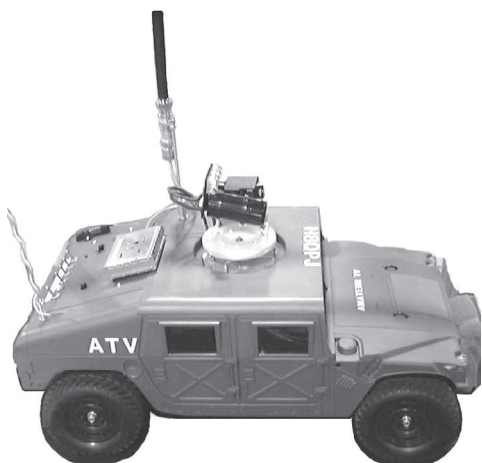
Fig 9.52 — N8QPJ mounted an ATV receiver aboard this model Humvee.
