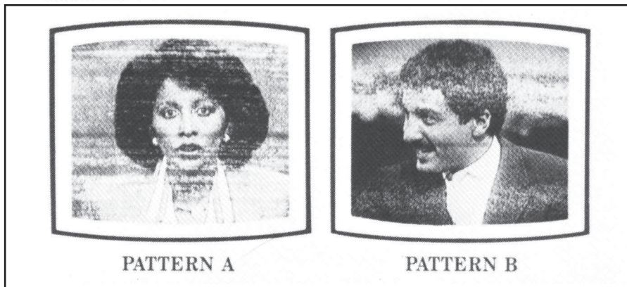
Fig 13.15 — Two examples of TVs experiencing electrical noise.
