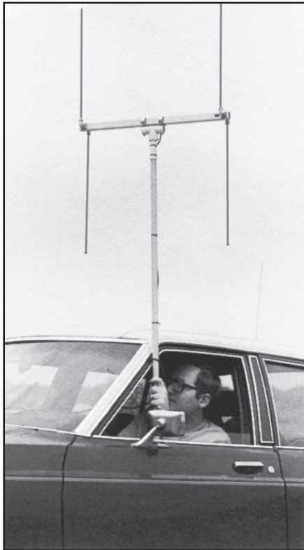
Fig 13.39 — A set of TDOA RDF antennas is light weight and mounts readily through a sedan window without excessive overhang.
