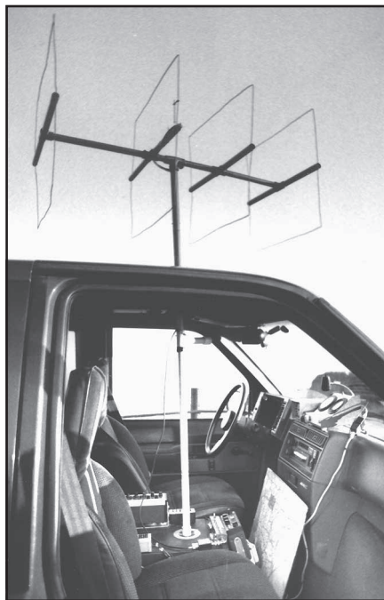
Fig 13.34 — K0OV uses this mobile setup for RDF on several bands, with separate antennas for each band that mate with a common lower mast section, pointer and 360° indicator. Antenna shown is a heavy gauge wire quad for 2 m.
