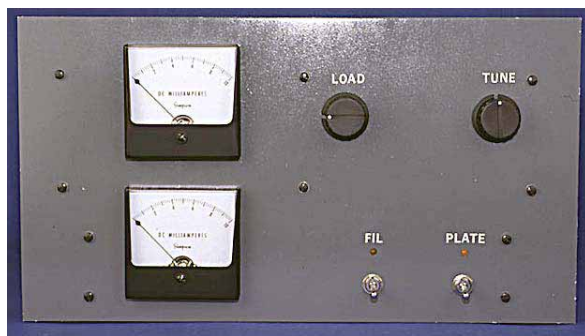
Fig 18.33 —Photo of the front panel of W1QWJ's 6-meter 4CX1600B amplifier.
