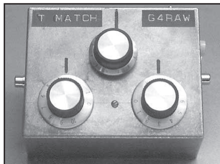
Fig 19.81 —The completed T-Match ATU.
