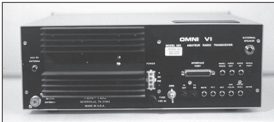
Fig 19.10 —The back of this Ten-Tec Omni VI HF transceiver shows some of the many types of connectors encountered in the amateur station. Note that this variety is found on a single piece of equipment. (Photo courtesy AA8DX)
