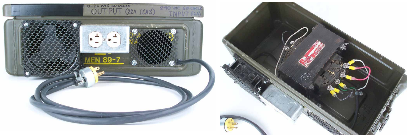
Fig 19.85 —W1LC’s Ugly Transformer project is contained in a surplus heavy-gauge-steel military ammo box. In the left photo, the small axial cooling fan, 20-A, 120-V ac outlet and fan exhaust vent can be seen, respectively, from left to right. The protective screening was from an old roll of “gutter guard” and is used to prevent accidental contact with components inside. Screening can be of either metallic or non-conductive construction. The photo at the right shows the control transformer and associated wiring inside with the cover off. Case grounding for electric mains purposes is accomplished by connecting the 240-V cord ground to a terminal securely fastened under one of the transformer’s mounting brackets. A stranded, insulated ground-wire jumper must also be connected between this grounding point and the cover to ensure a complete case ground. The use of a nylon cable clamp on the cord inside keeps it from being accidentally pulled out of the surplus enclosure.
