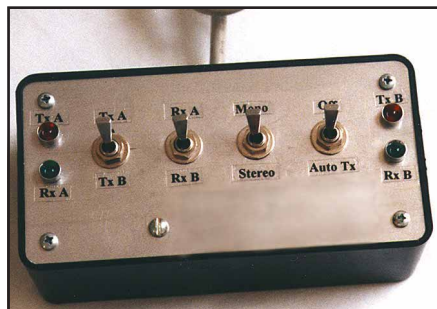
Fig 19.62—The remote head for the Two-Radio Switchbox.
