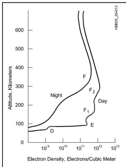
**Fig 20.13—Typical electron densities for the various ionospheric regions.**
