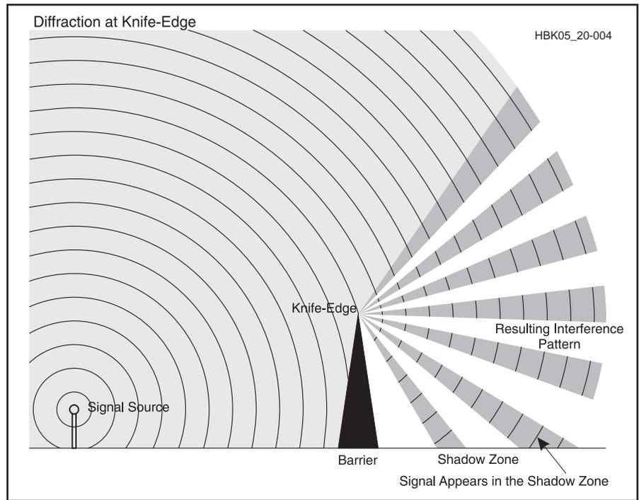
**Fig 20.4—Radio, light and other waves are diffracted around the sharp edge of a solid object that is large in terms of wavelengths. Diffraction results from interference between waves right at the knife-edge and those that are passing above it. Some signals appear behind the knife-edge as a consequence of the interference pattern. Hills or mountains can serve as natural knife-edges at radio frequencies.**
