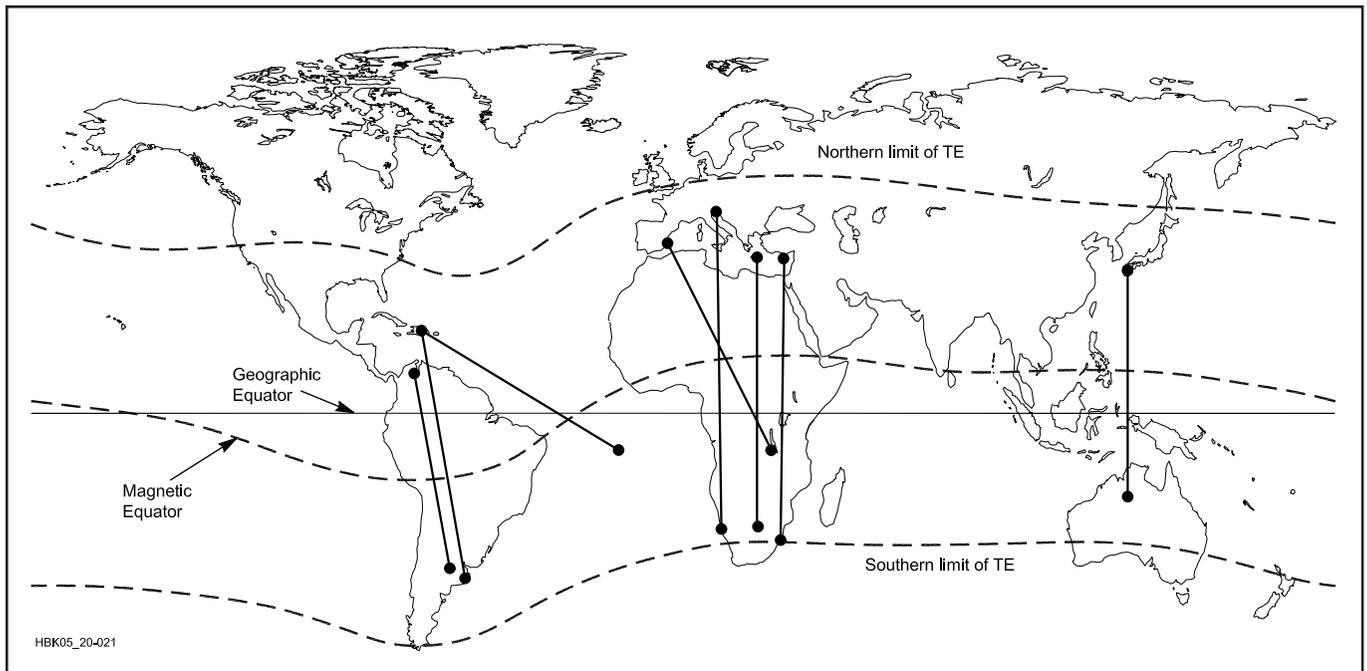
**Fig 20.21—Transequatorial spread-F propagation takes place between stations equidistant across the geomagnetic equator. Distances up to 8000 km (5000 mi) are possible on 28 through 432 MHz. Note the geomagnetic equator is considerably south of the geographic equator in the Western Hemisphere.**
