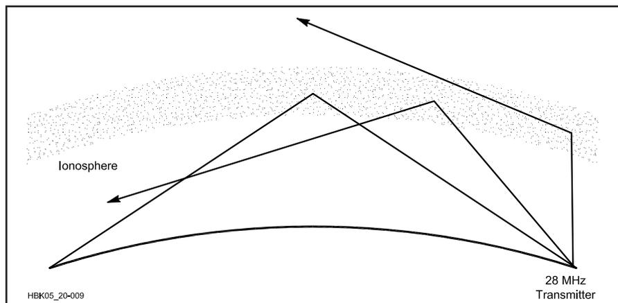
**Fig 20.9**—Signals at the MUF propagated at a low angle to the horizon provide the longest possible one-hop distances. In this example, 28-MHz signals entering the ionosphere at higher angles are not refracted enough to bring them back to Earth.
