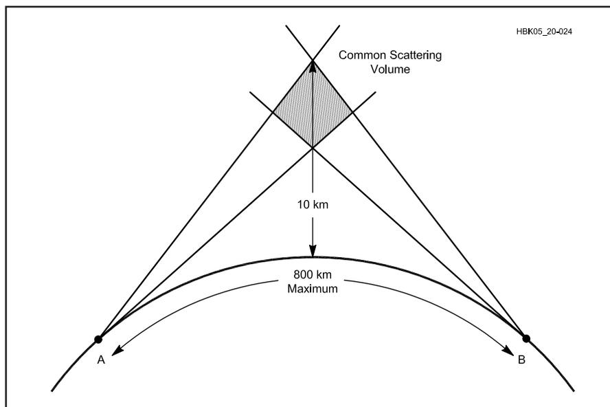
**Fig 20.24—Tropospheric-scatter path geometry.** The lower boundary of the common scattering volume is limited by the take-off angle of both stations. The upper boundary of 10 km (6 mi) altitude is the limit of efficient scattering in the troposphere. Signal strength increases with the scattering volume.
