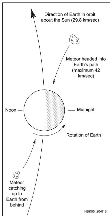
**Fig 20.16**—The relative velocity of meteors that meet the Earth head-on is increased by the rotational velocity of the Earth in orbit. Fast meteors strike the morning side of the Earth because their velocity adds to the Earth's rotational velocity, while the relative velocity of meteors that "catch up from behind" is reduced.
