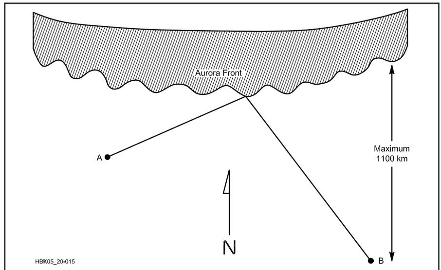
**Fig 20.15—Point antennas generally north to make oblique long-distance contacts on 28 through 432 MHz via aurora scattering. Optimal antenna headings may shift considerably to the east or west depending on the location of the aurora.**
