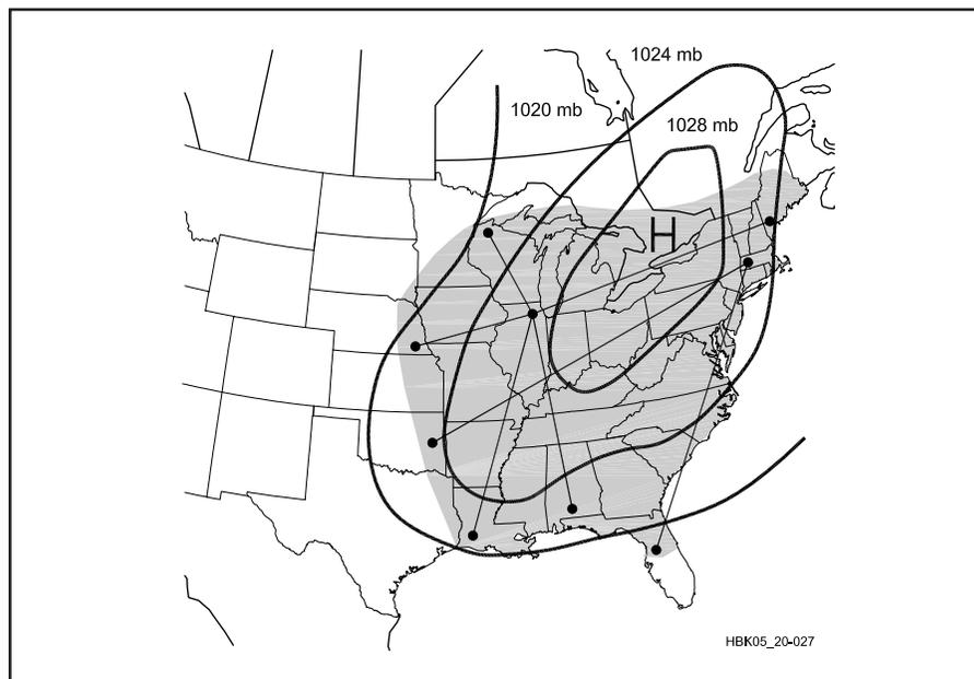
**Fig 20.27—Surface weather map for September 13, 1993, shows that the eastern US was dominated by a sprawling high-pressure system. The shaded portion shows the area in which ducting conditions existed on 144 through 1286 MHz and higher.**
