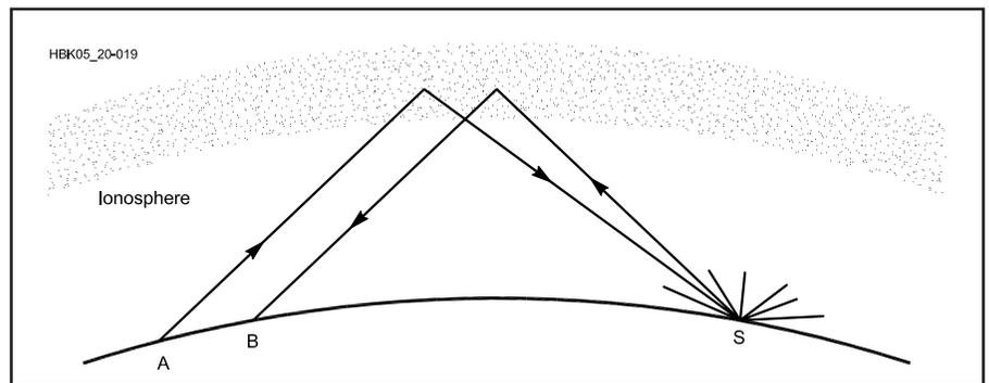
**Fig 20.19**—Schematic of a simple backscatter path. Stations A and B are too close to make contact via normal F-layer ionospheric refraction. Signals scattered back from a distant point on the Earth's surface (S), often the ocean, may be accessible to both and create a backscatter circuit.
