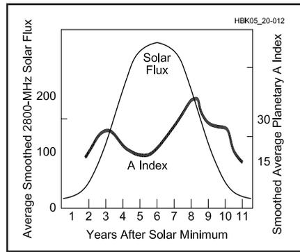
**Fig 20.12—Geomagnetic activity (measured as the A-index) also follows an 11-year cycle. Average values over the past few cycles show that geomagnetic activity peaks before and after the peak of solar flux.**
