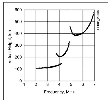
Fig 20.7—Simplified vertical incidence ionogram showing echoes returned from the E, F<sub>1</sub> and F<sub>2</sub> layers. The critical frequencies of each layer (4.1, 4.8 and 6.8 MHz) can be read directly from the ionogram scale.
