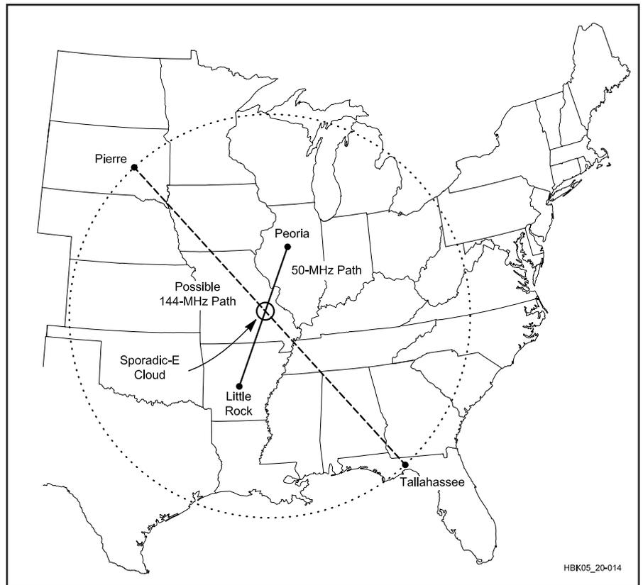
**Fig 20.14—50 MHz sporadic-E contacts of 700 km (435 mi) or shorter (such as between Peoria and Little Rock) indicate that the MUF on longer paths is above 144 MHz. Using the same sporadic-E region reflecting point, 144-MHz contacts of 2200 km (1400 mi), such as between Pierre and Tallahassee, should be possible.**
