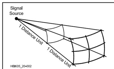
**Fig 20.2**—Radio energy disperses as the square of the distance from its source. For the change of one distance unit shown the signal is only one quarter as strong. Each spherical section has the same surface area.
