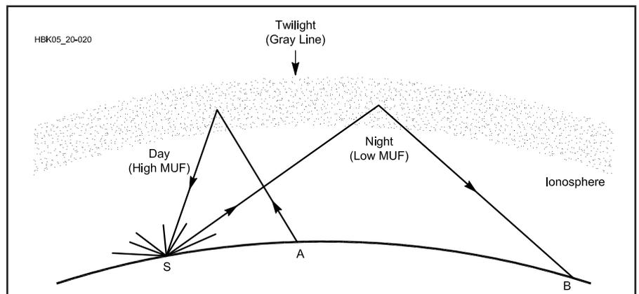
**Fig 20.20**—Backscatter path across the gray line. Stations A and B are too close to make contact via normal ionospheric refraction, but may hear each other's signals scattered from point S. Station A makes use of a high-angle refraction on the day side of the gray line, where the MUF is high. Station B makes use of a night-time refraction, with a lower MUF and lower angle of propagation. Note that station A points away from B to complete the circuit.
