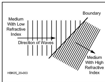
the refractive indices of two media is great enough, radio waves can be reflected, just like light waves striking a mirror. The Earth is a rather lossy reflector, but a metal surface works well if it is several wavelengths in diameter.
