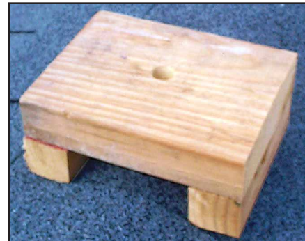
Fig 22.57 — At K8CH, the HVD base insulator sits in this saddle-shaped wooden fixture. This photo was taken before the fixture was painted—a necessary step to protect against the weather.
