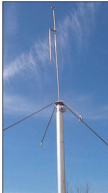
Fig 22.99 — WA3WMG's whip can be used to make a dual-band groundplane antenna. Separate radials for 2-m and 70-cm simplifies tuning. [Photo by K8CH]
