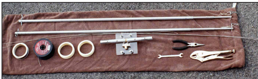
Fig 22.35 — The entire inverted-U antenna parts collection in semi-nested form, with its carrying bag. The tools stored with the antenna include a wrench to tighten the U-bolts for the mast-to-plate mount and a pair of pliers to help remove end wires from the tubing. The pliers have a wire-cutting feature to help replace a broken end wire. A pair of locking pliers makes a good removable handle for turning the mast. The combination of the locking and regular pliers helps to uncoil the wire extensions for any band; give them a couple of sharp tugs to straighten the wire.
