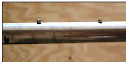
Fig 22.53 — Element splice uses a 1-ft length of 0.75-inch tubing inserted into the 0.875-inch sections to join them together. Self-tapping sheet-metal screws are used in this photo, but aluminum pop rivets or machine screws with washers and nuts can be used.
