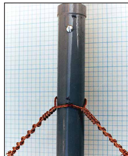
Fig 22.74 — Attaching quad wires to the spreaders must minimize stress on the wires for best reliability. This method (described in the text) cuts the chances of wind-induced wire breakage by distributing stress.
