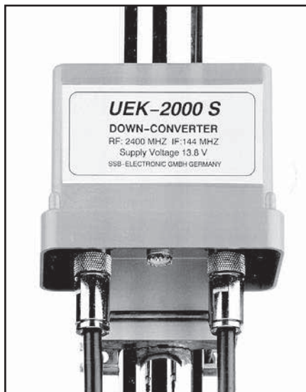
Fig 23.40 —This SSB Electronic unit (left) is one of several solutions for mast-mounted S-band receive converters. Other manufacturers, including Down East Microwave (top), have similar offerings.
