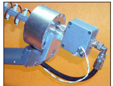
Fig 23.60—Mounting details of seven-turn helix and preamp.
