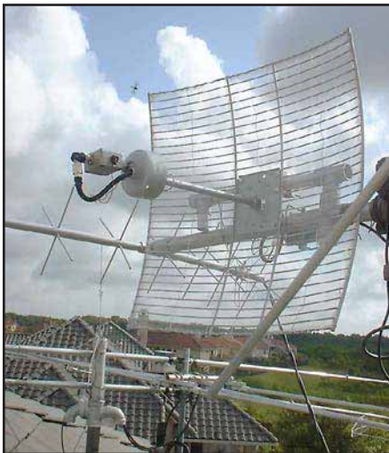
Fig 23.51 —K5OE's mesh modification of a MMDS dish antenna with helix CP feed and DEM preamp.
