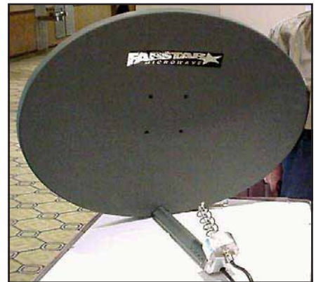
Fig 23.54 —PrimeStar offset-fed dish with WD4FAB's helix-feed antenna. N0NSV was so pleased with the modification that he renamed the dish "FABStar," and made a new label!
