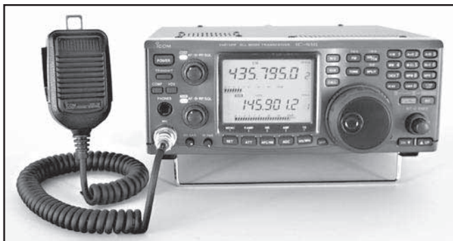
Fig 23.26 —ICOM's IC-910H, a recent entry into the multi band VHF/UHF transceiver world, has an available 23-cm module.
