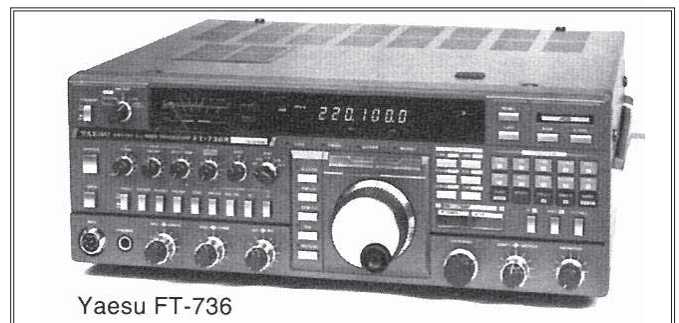
Fig 23.27 —The Yaesu FT-736R is a multimode transceiver for 2 m (144-148 MHz) and 70 cm (430-450 MHz). It can be used for full-duplex receiving and transmitting on AO-10 Mode U/V and AO-13 Modes U/V and V/U. An optional 23-cm module covers 1230-1300 MHz (Mode L/U). Approximate power output: 20 W on 2 m and 70 cm, and 10 W on 23 cm.
