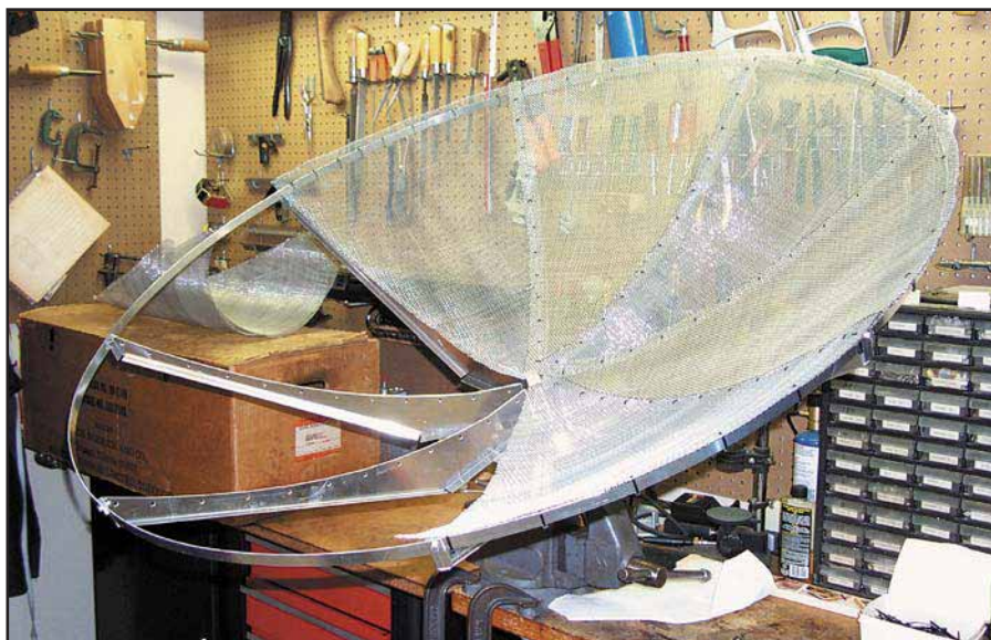
Fig 23.65—Dish antenna during assembly.
