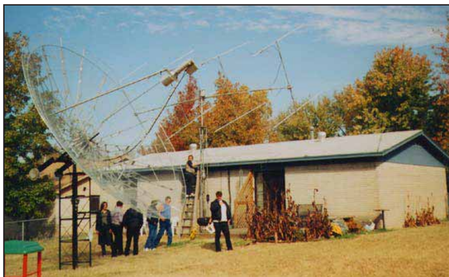
Fig 23.71—Tommy Henderson, WD5AGO, pursues 144-MHz EME from his Tulsa, Oklahoma, QTH with this array. Local electronics students helped with construction.
