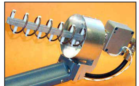
Fig 23.59—Seven-turn LHCP helix dish feed antenna with DEM preamp.
