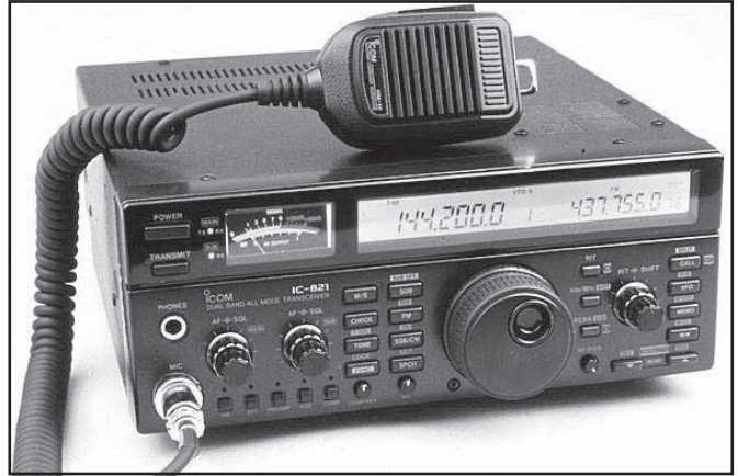
Fig 23.29 —ICOM’s IC-821H is another full-featured transceiver designed for satellite use.
