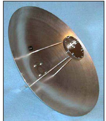
Fig 23.53 —G3RUH's 60-cm spun aluminum dish with CP patch feed, available as a kit.
