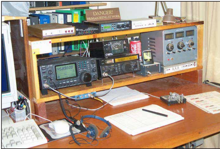
Fig 23.24 —WD4FAB's station is typical of a full-featured HF and satellite operation. On the bottom row, L-R are: IC-746 HF to 2 meter transceiver, IC-821H VHF-UHF multimode transceiver topped by a home-brew power meter, KLM 1200GU 1.2-GHz transverter, home-brew multi-antenna rotator controller on top of the station accessory control box. On the top row, L-R are: G3RUH AO-13 Telemetry Demodulator, PacComm SPIRIT2 high performance packet controller, Timewave DSP-599zx audio DSP unit for the VHF-microwave operations through the IC-821H and the TAPR EasyTrak antenna command unit for interfacing the computer tracking to the antenna controller.
