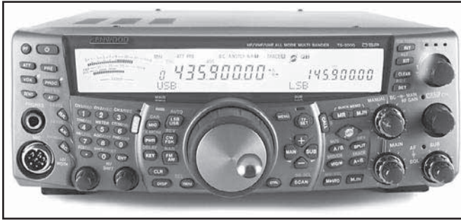
Fig 23.28 —Kenwood’s TS-2000 is an all-band, multimode transceiver that covers HF, 6 m, 2 m, and 70 cm. A 23-cm (1240-1300 MHz) module is optional. Typical power output is 35-45 W on 144 MHz, 30-40 W on 430 MHz and 10 W on 1240 MHz.
