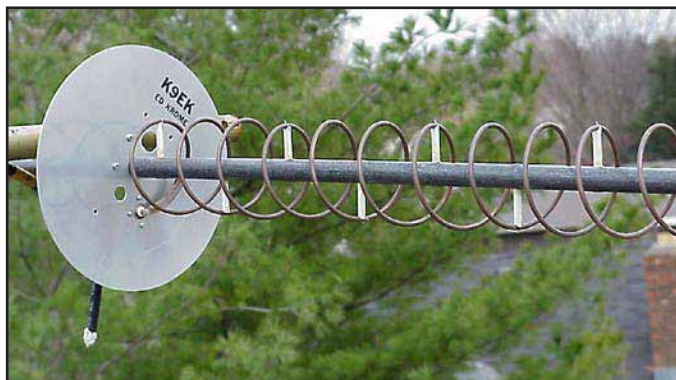
Fig 23.47—This L-band helix antenna was designed to be home-brewed without any special tools or shop equipment. It is mounted on a 4-foot-long fiberglass tube.
