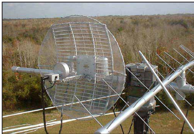
Fig 23.52 —K5GNA's "circularized" mesh modification of an MMDS dish antenna with helix CP feed and DEM preamp.
