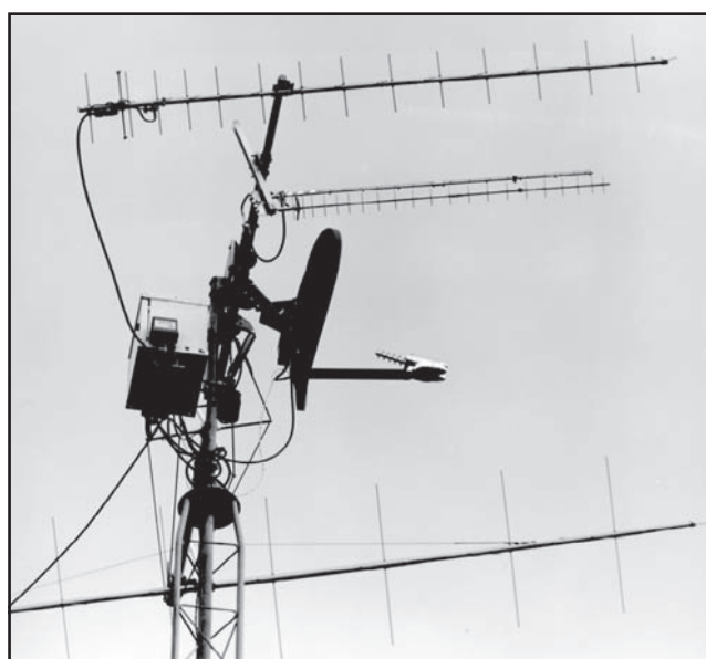
Fig 23.41 —Details of WD4FAB’s tower cluster of satellite antennas, including a home-brew elevation rotator. Top to bottom: M2 436-CP30, a CP U-band antenna; two each M2 23CM22EZA antennas shown in a CP array for L band; “FABStar” dish antenna with helix feed for S band; M 2 2M-CP22, a CP V-band antenna (only partially shown.) To left of dish antenna is a NEMA4 equipment box with an internal 40W L-band amplifier, and also hosts externally-mounted preamplifiers.
