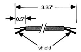
[] Install W1 and W2. The center conductor at each end of W1 goes to a point labeled "W1," while the shield at each end of W1 goes to the nearest ground point. (Every point intended for a jumper has a white "donut" symbol on the silkscreen.) W2 is installed in a similar fashion. You can install the coax jumpers on either the top or bottom of the board. If you install the jumpers on the bottom of the board, be careful not to let the shield leads short to any other traces.
