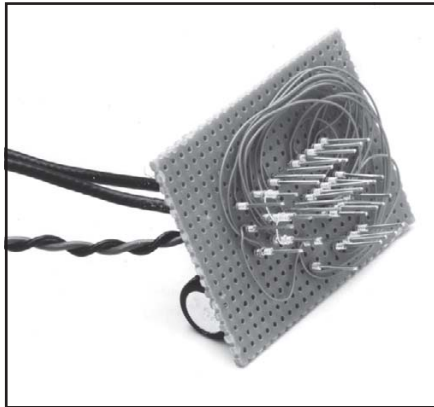
Fig 8.17—The audio amplifier built using wire-wrap techniques.
