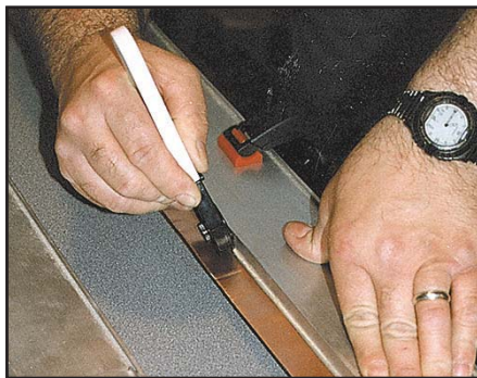
Fig 17.36 — Larry Wolfgang, WR1B, using a 4-foot straightedge designed as a guide for hand-held circular saws to clamp the copper-foil tape to a board on a tabletop. After carefully measuring to ensure a uniform 22-mm width, he cut the foil tape using a Fiskars rotary cutter. Be careful to keep the cutter wheel against the straightedge for the entire length. Move the tape in 4-foot intervals to cut the entire length. (Photo by Dan Wolfgang.)
