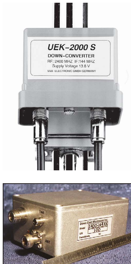
Fig 23.36 —This SSB Electronic unit (left) is one of several solutions for mast-mounted S-band receive converters. Other manufacturers, including Down East Microwave (top), have similar offerings.
