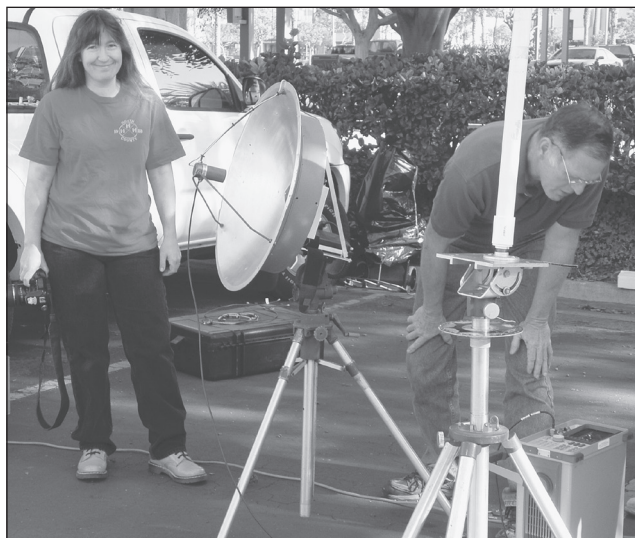
Fig 1.9 — Hams enjoy building and comparing antennas — all the way up to the microwave bands! In this photo from the 2010 Microwave Update convention, Kerry Banke, N6IZW (right) is measuring the performance of the 5.7 GHz dish built by Michelle Thompson, W5NYV. (W1GHZ photo)
