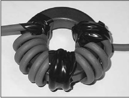
**Fig 5.38** — A ferrite choke consisting of multiple turns of cable wound on a 2.4-in. OD  $\times$  1.4-in. ID  $\times$  0.5-in. toroid core.
