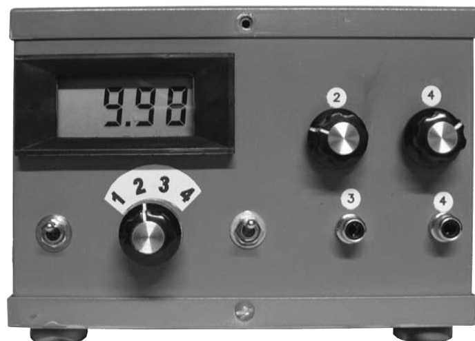
Fig 7.58 — The front panel of the four-output switching supply.
