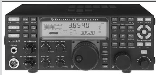
Fig 12.A4 — The Elecraft K3. It looks like a traditional amateur transceiver, but is actually an SDR.
