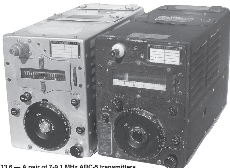
Fig 13.6 — A pair of 7-9.1 MHz ARC-5 transmitters from WW2. On the left the US Army Air Forces version (BC-459), on the right a Navy equivalent (T-22, ARC-5). These were available for typically $5 in "new in box" condition after WW2.
