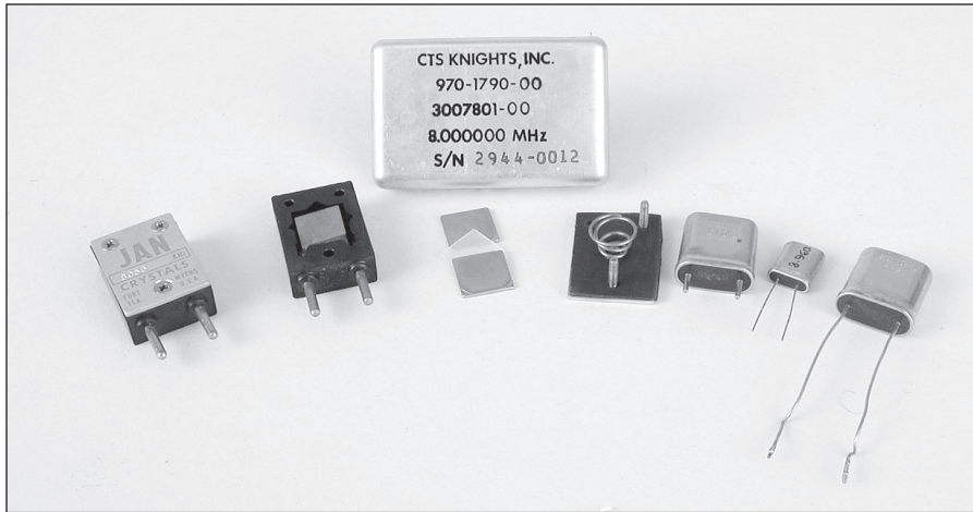
Fig 13.7 — Sample of typical frequency control crystals for amateur use. The units on the right are modern sealed types. On the far left is a WWII era crystal with a disassembled holder in the center.
