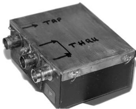
Fig 14.17 — Sample of a box made with PC board with a sheet brass cover overlapping all four sides. Note the BNC connectors and feed thru insulator.
