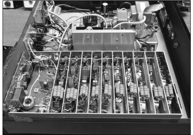
Fig 14.21 — The 100-W amplifier, 10 low-pass filters and the power supplies are located in a separate enclosure.
