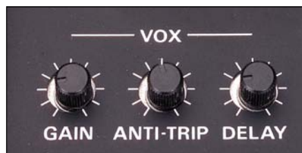
Fig 14.9 — The function of VOX controls is described in the text. They require adjustment for different types of operating, so front-panel knobs make the most convenient control arrangement. In some radios, VOX settings are adjusted through the menu system.
