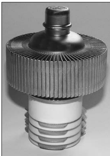
Fig 17.9 — Modern power tubes, such as this 4CX1000A tetrode, tend to use metal and ceramic construction.
