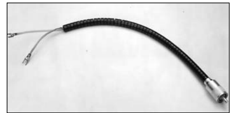
Fig 20.30 — W2DU bead balun consisting of 50 FB-73-2401 ferrite beads over a length of RG-303 coax. See text for details.
