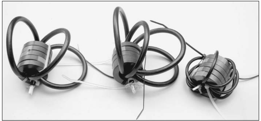
Fig 20.26 — Typical transmitting wound-coax common-mode chokes suitable for use on the HF ham bands.
