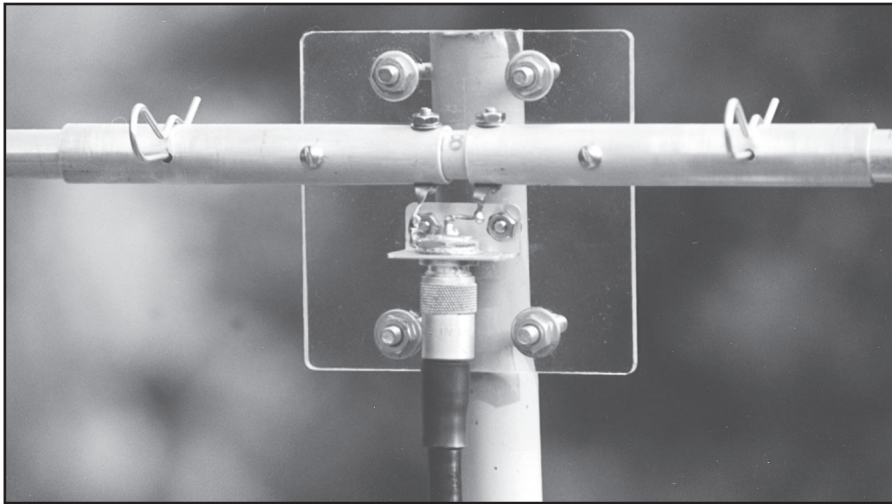
Fig 21.35 — A close-up of the element mounting plate assembly, including the hitch pin clips used to secure the next section of tubing.
