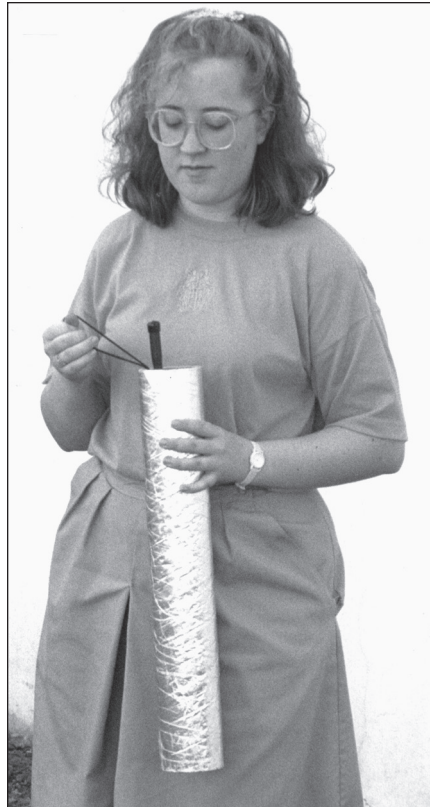
Fig 21.145 — The air attenuator for a VHF hand-held in use. Suspend the radio by the wrist strap or a string inside the tube.
