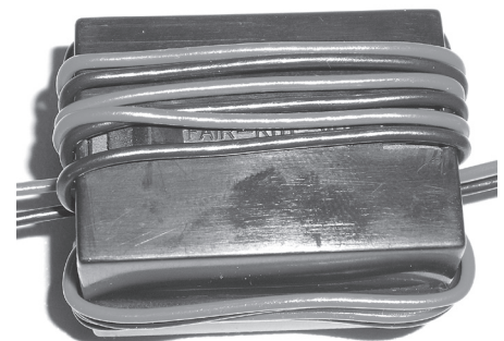
Fig 21.96 — RF choke for screwdriver antenna control and power leads.
