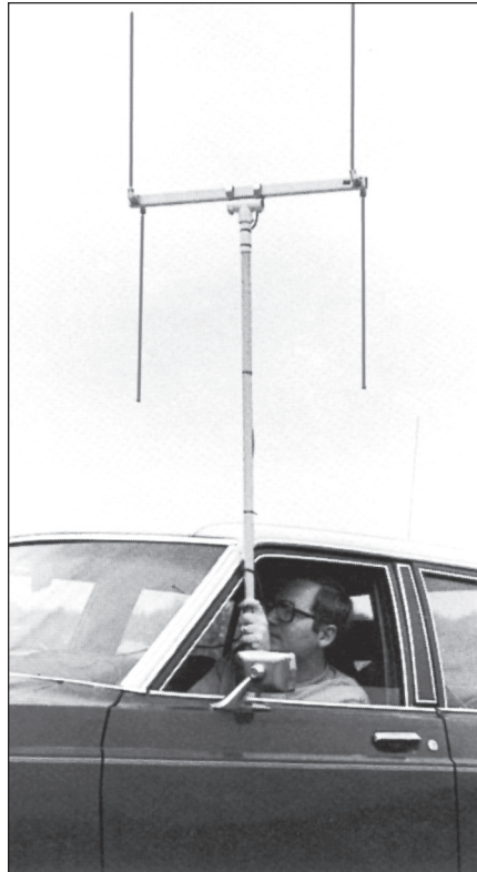
Fig 21.139 — A set of TDOA RDF antennas is light weight and mounts readily through a sedan window without excessive overhang.
