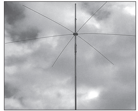
Fig 21.53 — W9SR's short vertical uses top loading and a capacitance hat with a 10-ft TV mast to make a compact antenna for 160, 80 or 40 meters.
