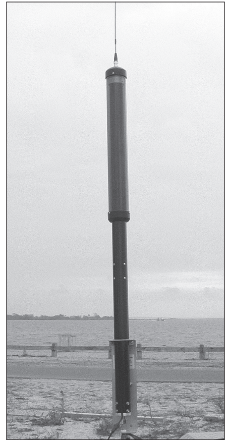
Fig 21.95 — The screwdriver-style remotely-controlled whip antenna. A small motor in the base mast moves a coil past contacts at the top of the metal base section. The top whip section is attached to the top of the coil. As the coil moves out of the mast, more inductance is connected in series between the base section and top section. Screwdriver antennas are popular because they offer multiband coverage. (W1ZR photo)
