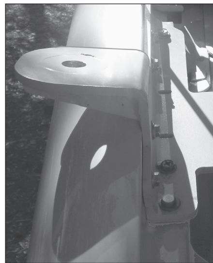
Fig 21.102 — The KE5DKM bracket mounts under the hood of a motor home.
