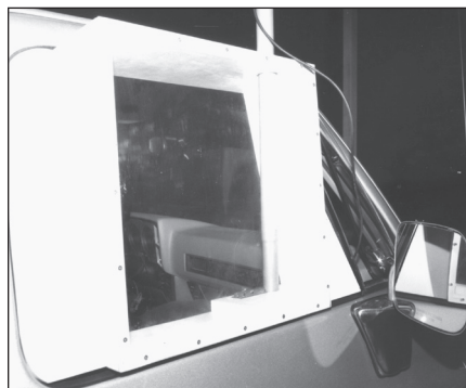
Fig 21.140 — A window box allows the navigator to turn a mast mounted antenna with ease while remaining dry and warm. No holes in the vehicle are needed with a properly designed window box.
