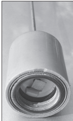
Fig 21.104 — The NMO (New Motorola) mount is widely used for VHF and UHF mobile antennas. It is available in mag-mount, trunk and lip mount and through-body mounting styles.
