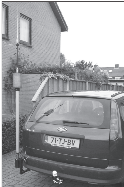
Fig 21.100 — The PA3VOS antenna mount easily supports a large screwdriver antenna and is offset to allow the hatch to open and close without removing the antenna.
