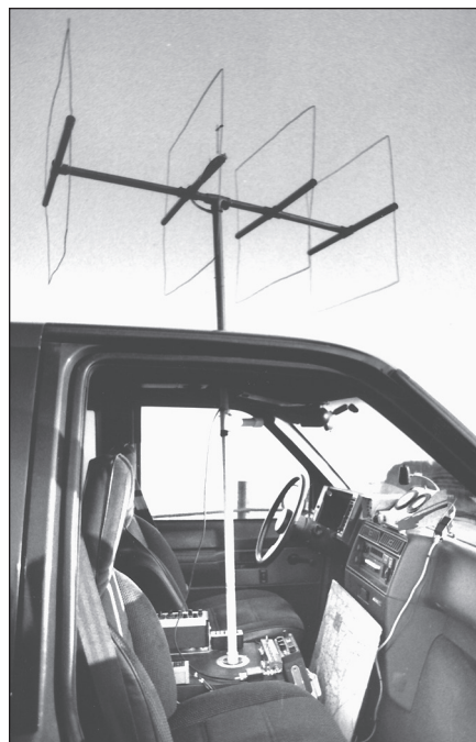
Fig 21.134 — K0OV uses this mobile setup for RDF on several bands, with separate antennas for each band that mate with a common lower mast section, pointer and 360° indicator. Antenna shown is a heavy gauge wire quad for 2 meters.
