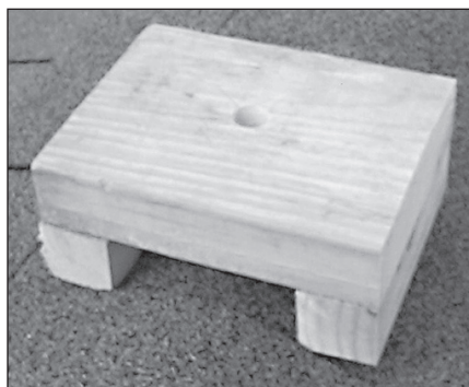
Fig 21.64 — At K8CH, the HVD base insulator sits in this saddle-shaped wooden fixture. This was photo was taken before the fixture was painted—a necessary step to protect against the weather.
