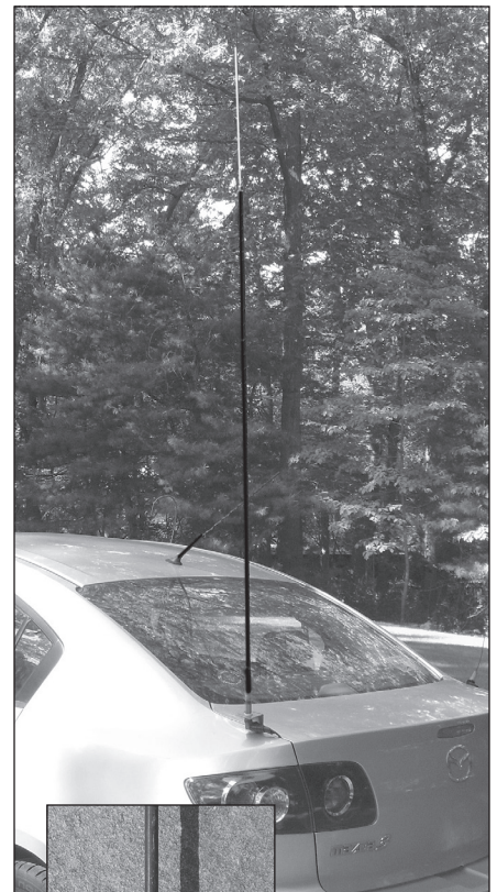
Fig 21.94 — Continuously-loaded whip antennas are short and lightweight. The base section consists of a fiberglass tube wound with wire to form the loading inductor. At the top of the base section the length of a steel whip or stinger can be adjusted to bring the antenna to resonance. (W1ZR photo)
