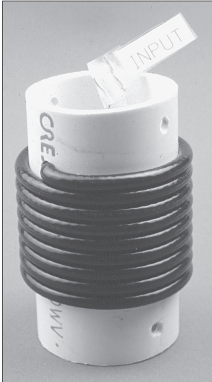
Fig 21.45 — Additional construction details for the W8NX coax-cable trap.
