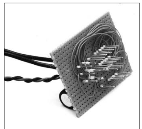
Fig 23.13 — The audio amplifier built using wire-wrap techniques.
