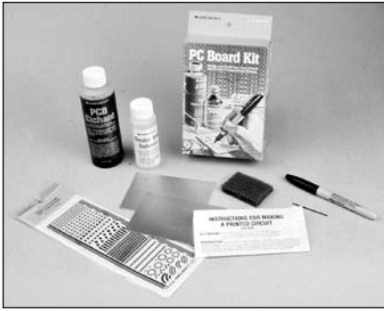
Fig 23.18 — PC-board materials are available from several sources. This kit includes layout materials, etchant, and PC board stock.
