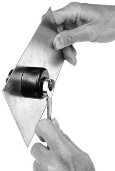
Fig 23.3 — A socket punch is used to easily punch a hole in sheet metal.
