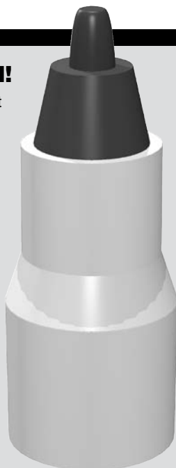
Fig 23.A9 — Make a permanent marker into a specialized PC-board drawing tool. Simply press the marker point into a drilled hole to form a modified point as shown. More pressure produces a wider shoulder that makes larger pads on the PC board.
