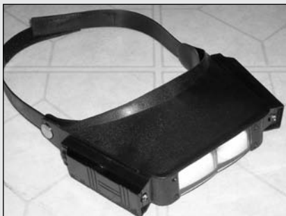
Fig 23.A2 — A magnifying visor is great for close-up work on a circuit board. These headsets are often available for less than $10 at hamfests and some even come with superbright LEDs mounted on the side to illuminate the components being soldered.
