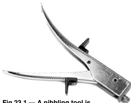
Fig 23.1 — A nibbling tool is used to remove small sections of sheet metal.
