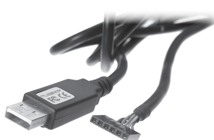
Fig 24.40 — The FTDI TTL-232R cable simplifies construction.
