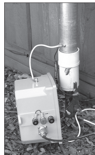
Fig 24.16 — The finished matching unit at the base of the author's 43-ft antenna (strapped for 80 meter operation).
