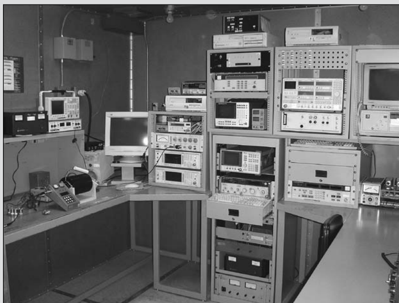
The ARRL Lab maintains an RF-tight screen room with a full suite of equipment for Product Review testing.
