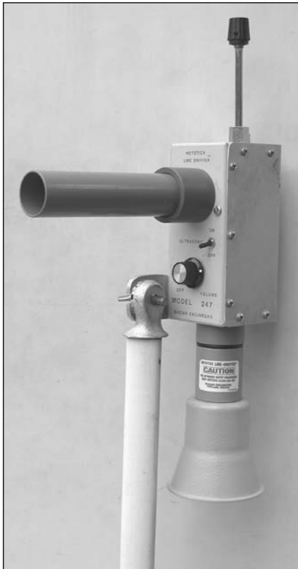
Fig 27.11 — The Radar Engineers Model 247 Hotstick Line Sniffer is an RF and ultrasonic locator. It is used by utility workers to pinpoint the exact piece of hardware causing a noise problem. Mounted on a hotstick, the sniffer is used from the pole or from a bucket.
