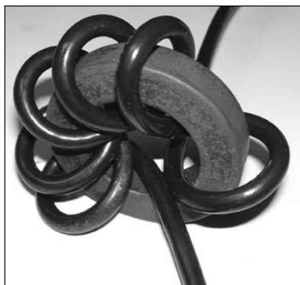
Fig 27.20 — To eliminate HF and VHF signals on the outside of a coaxial cable, use an 1- to 2-inch OD toroid core and wind as many turns of the cable on the core as practical.
