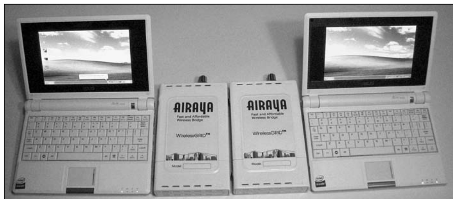
Fig 29.33 — Solid-state disk drives in netbook-style computers and wireless point-to-point Ethernet bridges can be used to form a low-power, high-reliability computer-to-computer control link.
