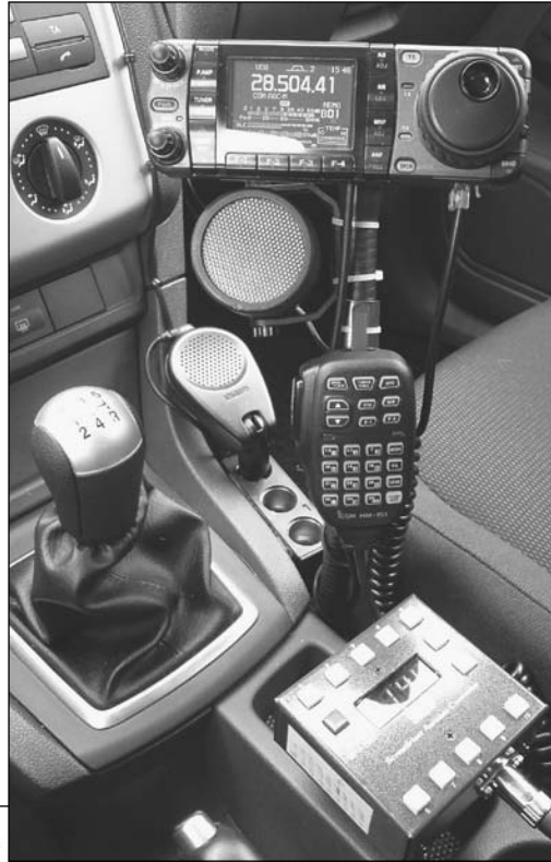
Fig 29.18 — At A, the transceiver control head is attached to one of many available mounts designed for this purpose. Mounts are typically highly adjustable, allowing the control head or radio to be positioned close to the operator. An antenna controller is mounted below the microphone. At B, HF and VHF transceiver control heads and the microphone are all mounted to the dashboard, within easy reach.
