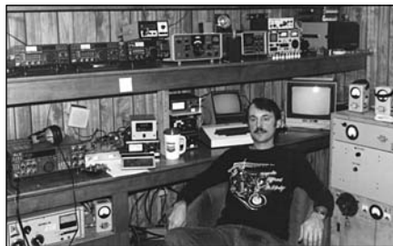
Fig 29.8 — Richard, WB5DGR, uses a homebrew 1.5-kW amplifier to seek EME contacts from this nicely laid out station.
