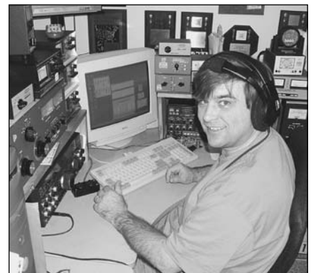
Fig 29.1 — Randy, K5ZD, has arranged his equipment for efficient contest operation. The computer keyboard and monitor occupy center stage, flanked by two transceivers and amplifiers and various accessories and control switches. (Photo courtesy Andrew Thompson)
