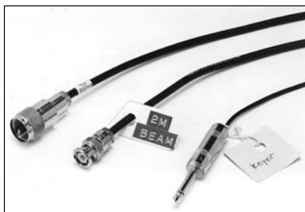
Fig 29.9 — Labels on the cables make it much easier to rearrange things in the station. Labeling ideas include masking tape, cardboard labels attached with string and labels attached to fasteners found on plastic bags (such as bread bags).
