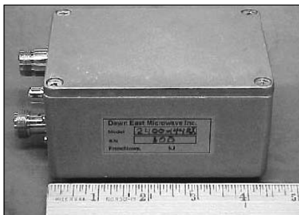
Fig 34 — This downconverter by Down-east Microwave converts signals at 2.4 GHz to 2 m. With its weatherproof enclosure, it is designed to be installed at the antenna.
