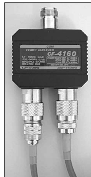
Fig 19 — A diplexer made by the Comet Corporation. Diplexers can be used to separate or combine signals on different bands.
