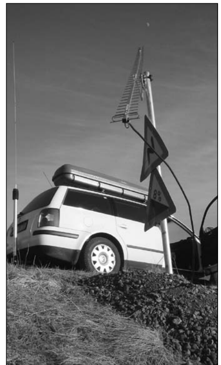
Fig 66 — TF/DL3OCH used a rural road sign to help him give contacts with Iceland to a number of EME operators on 1296 MHz. Bodo has activated many DXCC entities on 1296 MHz EME by using JT65, a single long Yagi and a 100 W solid state amplifier.
