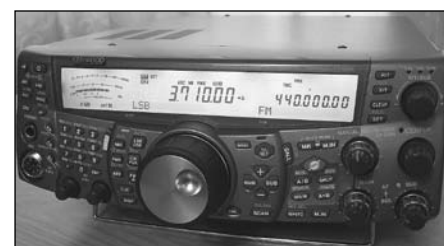
Fig 40 — The Kenwood TS-2000 offers full HF coverage, plus VHF and UHF with full-duplex satellite capability.
