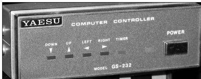
Fig 30 — The Yaesu GS-232 allows your computer and satellite tracking software to automatically control the movements of compatible azimuth/elevation antenna rotators.
