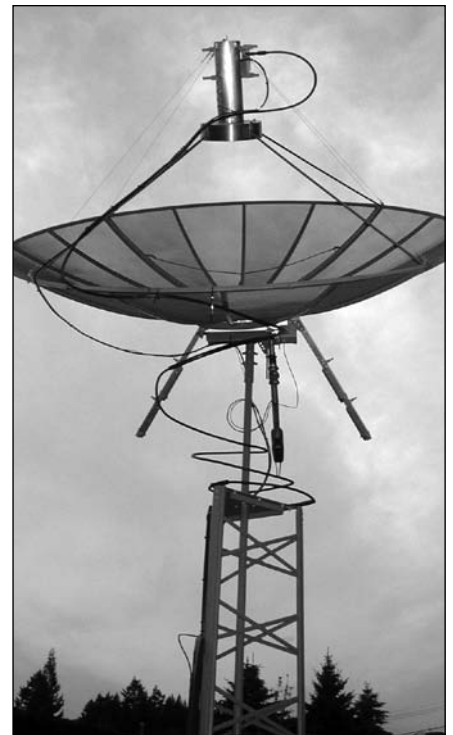
Fig 70 — This 3 m TVRO dish with aluminum frame and mesh surface was outfitted for 1296 MHz EME as a joint effort by VA7MM and VE7CNF. The dual-circular polarization feed is a VE4MA/W2IMU design.
