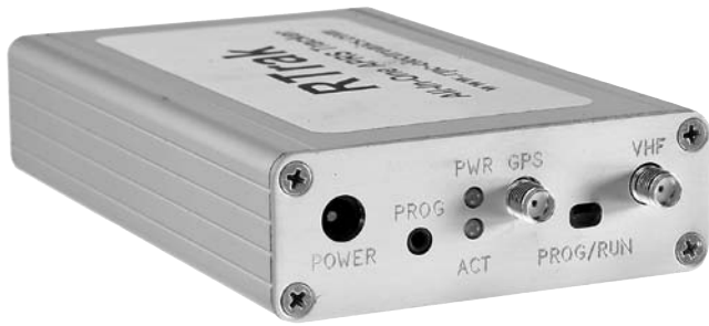
Fig 12 — Some APRS position encoders, such as this RPC Electronics RTrak, combine the GPS receiver, packet circuitry and 2 meter transmitter into a single device.
