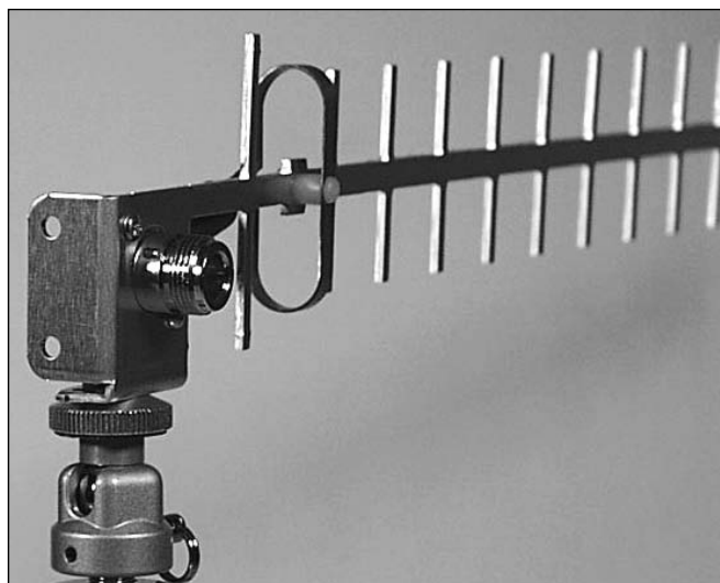
Fig 21 — Directional antennas, such as this MFJ 2.4 GHz Yagi, are best for HSMM links.
