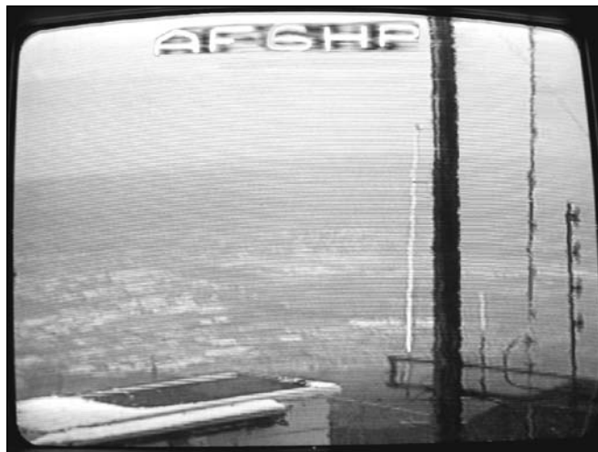
Fig 15 — ATV repeater “tower cam” IDs have become popular so that users can see approaching weather. Some cameras have remote pan and tilt, so users can observe ice build-up on antennas or activity at the repeater site.
