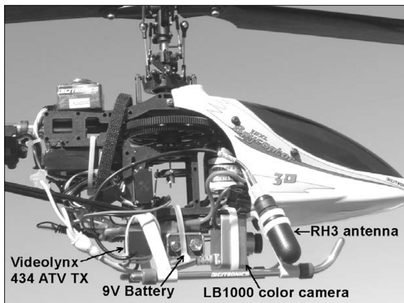
Fig 19 — At A, cable ties are used to fasten an LB-1000 color camera, Videolynx 434 ATV transmitter, 9-V battery and Diamond RH3 antenna to an R/C helicopter powered by an electric motor. At B, a computer with a TV tuner plugged into the USB port is used to view video coming from the ATV transmitter on the R/C helicopter — in this case, looking back at the R/C model operator.
