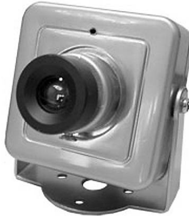
Fig 25 — The tiny LB-1000 420-line CMOS color camera is typical of the many low-cost devices available. Intended primarily for security applications, they are popular with amateurs.
