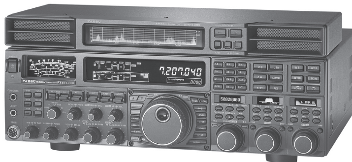
Fig 21 — The Yaesu FTDX5000 is one of a family of top-performing 200 W transceivers expandable with a 300 Hz roofing filter and multiple display options. The unit on top is the companion SM-5000 station monitor.
