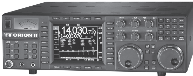
Fig 20 — The Ten-Tec Orion II offers excellent receive dynamic range through very narrow HF roofing filters in its main receiver.
