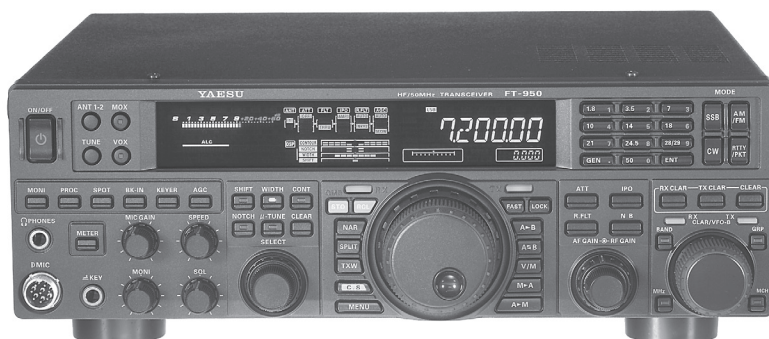
Fig 14 — The Yaesu FT-950 HF and 6 meter transceiver provides most of the FT-2000 functionality except the second receiver.
