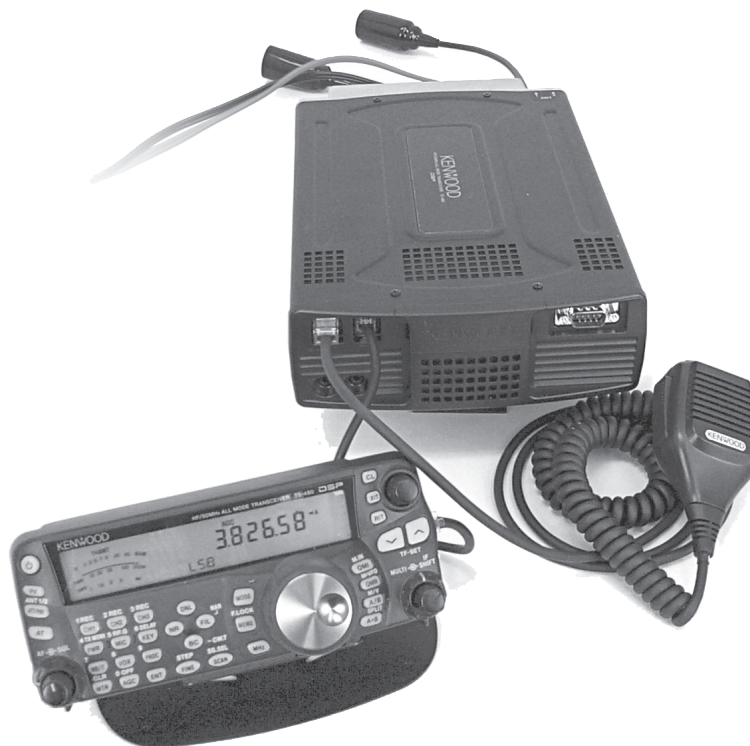
Fig 6 — Kenwood TS-480HX, the only transceiver in this category with a 200 W transmitter. The TS-480SAT looks similar, but offers 100 W output and an internal antenna tuner.
