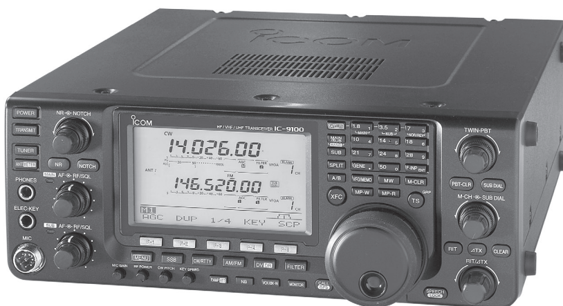
Fig 16 — The ICOM IC-9100H transceiver offers coverage of 1.8 through 440 MHz with an option for 1.3 GHz operation.
