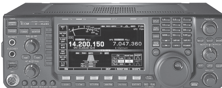
Fig 19 — The ICOM IC-7600 transceiver provides improved receiver performance through included 3, 6 and 15 kHz roofing filters.
