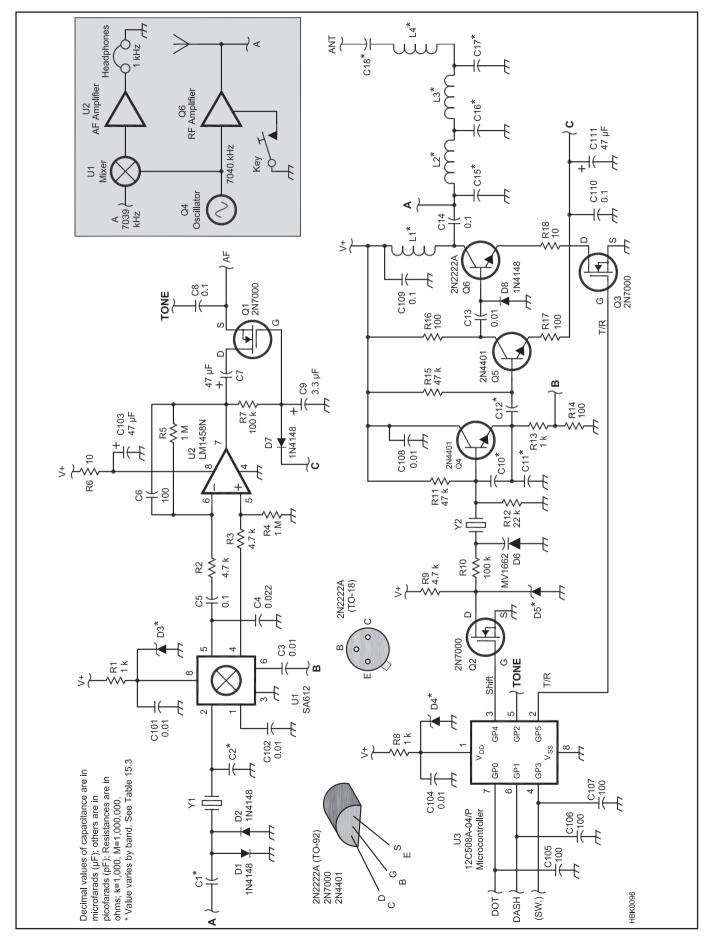
Fig 15.12 — The RockMite transceiver simplified block diagram (inset) and schematic. Most components are stocked by major distributors such as Digi-Key, Mouser and Ocean State Electronics (see the *TISFind* database at www.arrl.org/tis). Resistors are 5% <sup>1</sup>/<sub>4</sub> W. C1, C2, C10, C11, C12, C18 — NP0 disk
