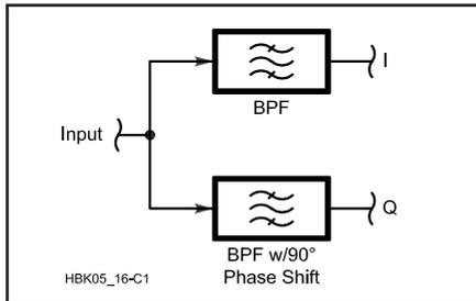
Fig 16.C1—Hilbert transformer using an analytic filter pair.
