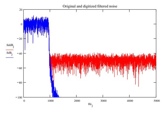
With an 8-bit quantizer, the quantization noise should theoretically be  $SNR_{eff} = 1.76 + 8 * 6.02 + 10 log(10,000/(2*1000)) = 56.9 dB$ .
