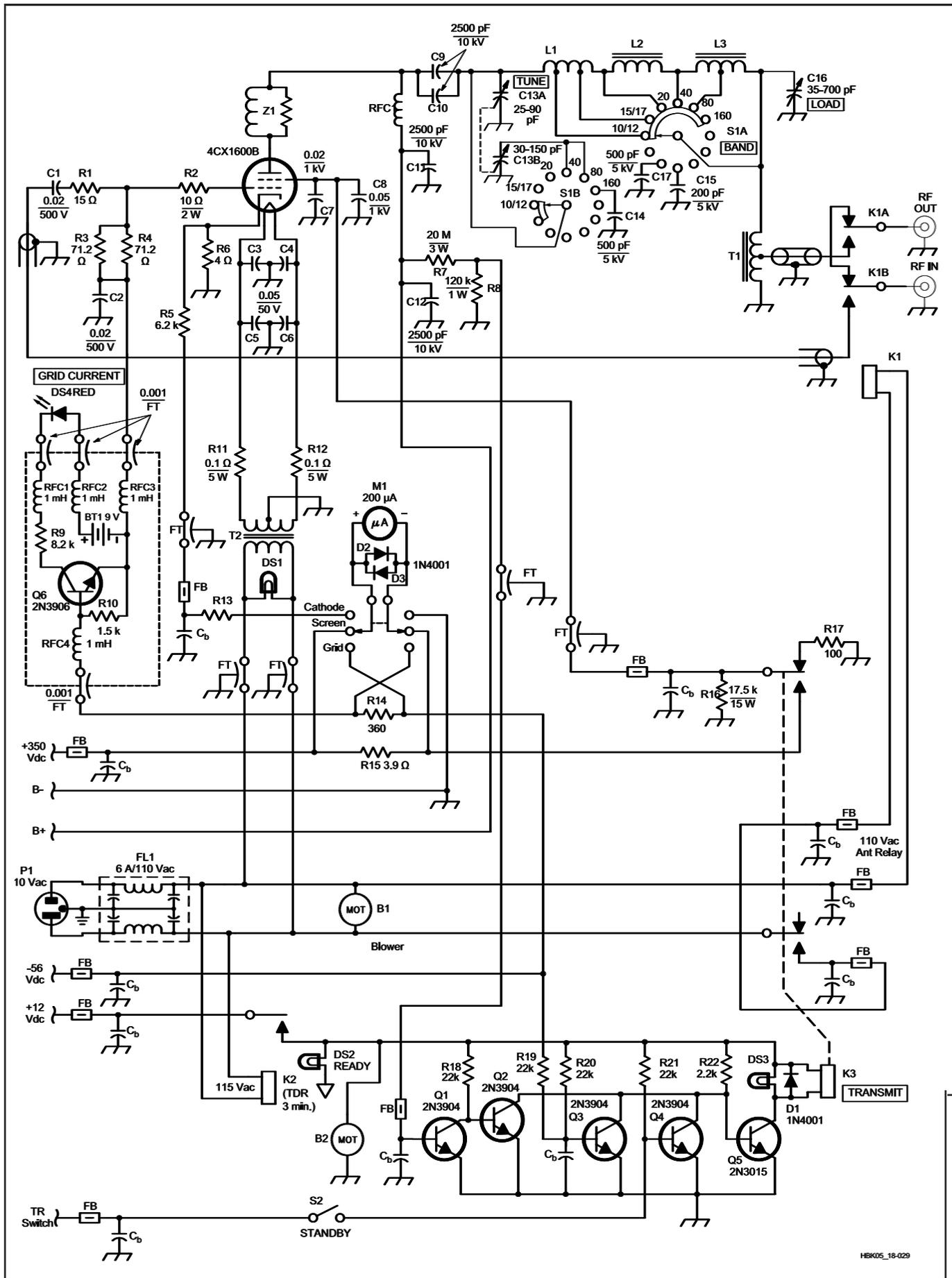
**Fig 18.29—Schematic diagram of the RF Deck of the 4CX1600B linear amplifier. Resistors are 1/2 W unless noted. Capacitors are disc ceramic unless noted and those marked with a + are electrolytic.**
