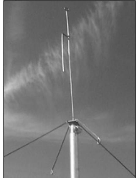
Fig 21.111 — K3MF's whip can be used to make a dual-band ground-plane antenna. Separate radials for 2 meters and 70-cm simplifies tuning. (Photo by K8CH)
