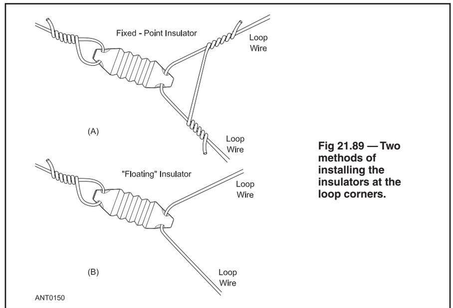
Fig 21.89 — Two methods of installing the insulators at the loop corners.
